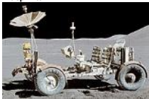
Lunar Roving Vehicle flown on Apollo 15
